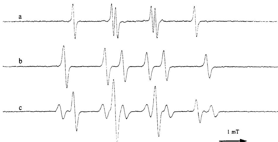
FIGURE 2 ESR spectra of spin adducts of CIMO with hydroxyl (a), carbon-centered radical (b) and DMPO adducts (c) generated by Fenton's reagent in the presence of 10% (v/v) EtOH (experimental conditions according to footnote of Tab. 1, receiver gain, 5 \cdot 10^4 )
