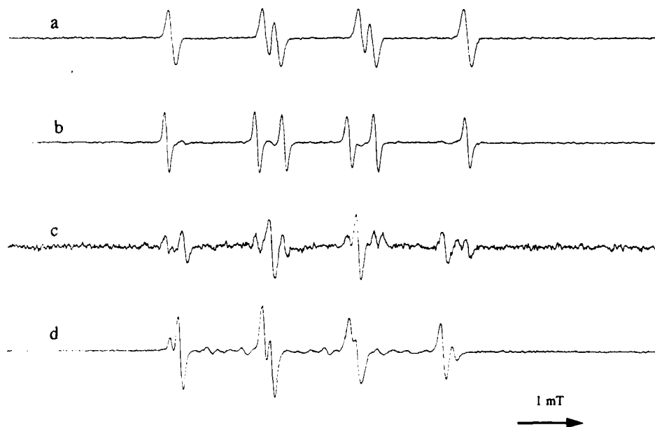
FIGURE 4 ESR spectra of sulfite radical adducts of DMPO (a), CIMO (b) and adducts formed with CIMO in solutions of bisulfite (c) and after UV-photolysis of persulfate (d) (experimental conditions according to footnote of Table 1, receiver gain, 5 \cdot 10^4 [a, b, d], 2 \cdot 10^5 [c])
